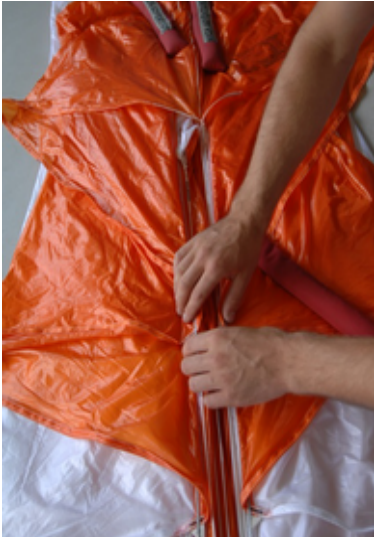
Fig. 68 check free run of the lines...
