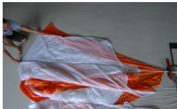
Fig. 32 fasten the line of panel No. 1 in the line separator. Fig. 33 spread out panel No. 1. Caution: make sure that the line is on top of the middle lines, which forms the axis of the reserve. Shape and size of this panel can vary depending on the brake configuration.
