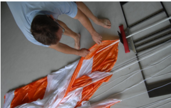
Fig. 30 pick up the trailing edge starting at the middle line
