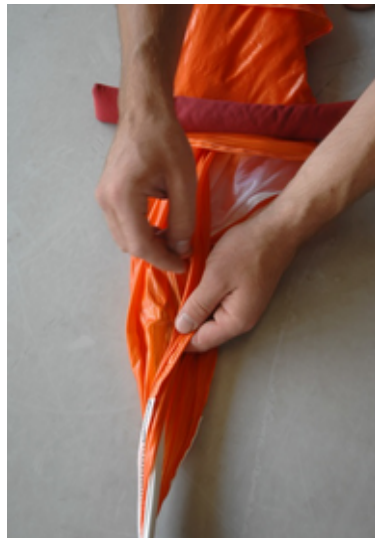
Fig. 82-84 wrap panel No. 1 around all the lines...
