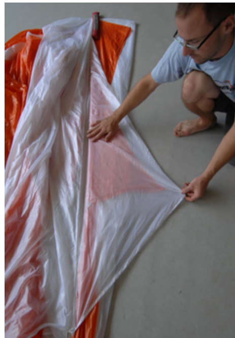
Fig. 37 lay the second panel on top of the first
