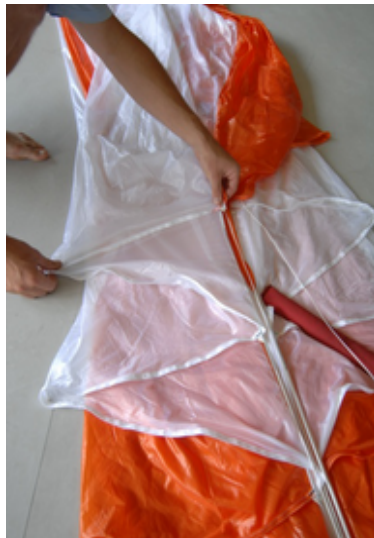
Fig. 66 folding of the second side is identical to the first one
