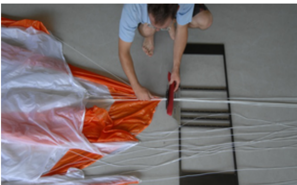
Fig. 32 fasten the line of panel No. 1 in the line separator. Fig. 33 spread out panel No. 1. Caution: make sure that the line is on top of the middle lines, which forms the axis of the reserve. Shape and size of this panel can vary depending on the brake configuration.
