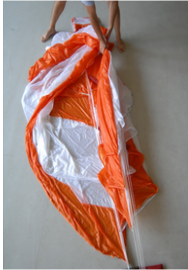
Fig. 63-64 put opposite half of the wing including lines over the line separator to the other side
