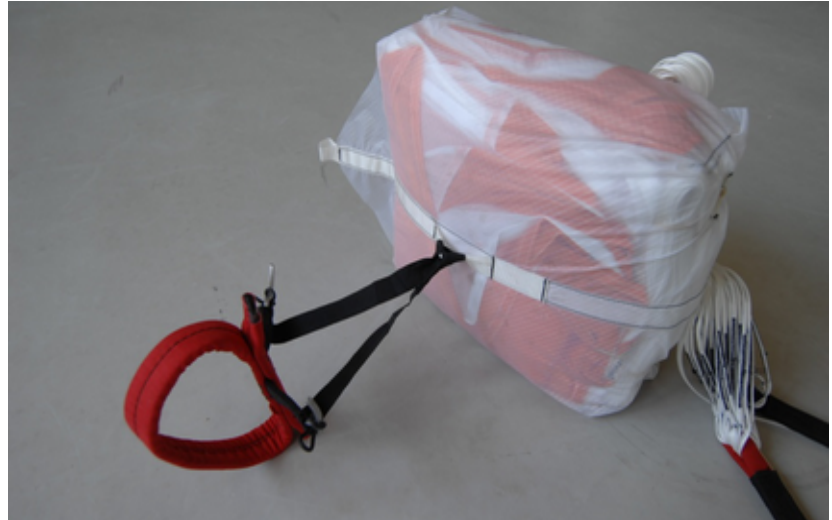
Fig. 112 Attachment of handle when using front container
