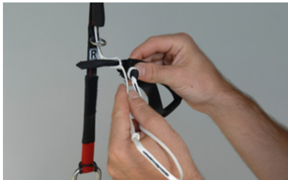
Fig. 4 Stowing the brake line for opening with brakes applied. Shoulder attachment of the reserve parachute.
