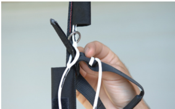
Fig. 3 Stowing the brake line for opening with brakes applied. Front attachment of the reserve parachute.
