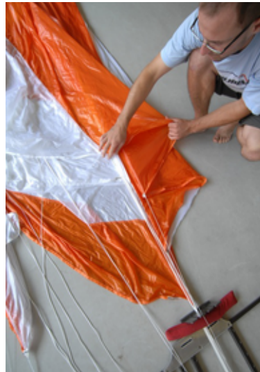
Fig. 51-52 folding of subsequent panels (as far as the wing tip) is carried out according to the description on folding panels 3, 4 and 5
