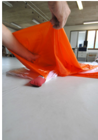
Fig. 48-49 sweep panel No. 4 outwards (s-fold)
