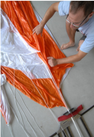
Fig. 50 anchor the line of panel No. 5 to the line separator
