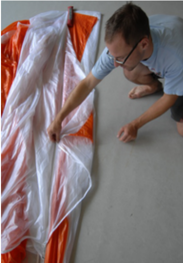
Fig. 38 reduce panel No. 2 by s-fold
