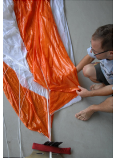
Fig. 45-46 anchor the line of panel No. 4 to the line separator
