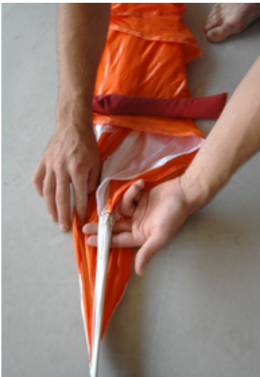
Fig. 82-84 wrap panel No. 1 around all the lines...
