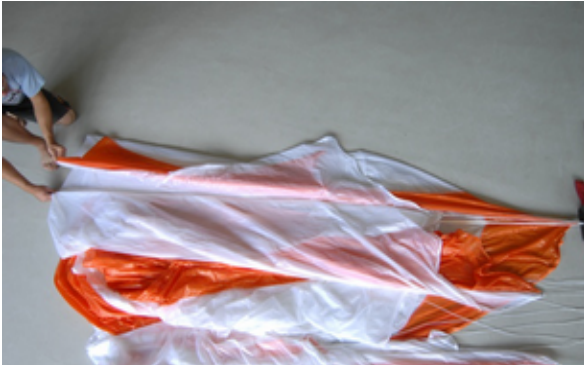
Fig. 34 reduce panel No. 1 using a double s-fold
