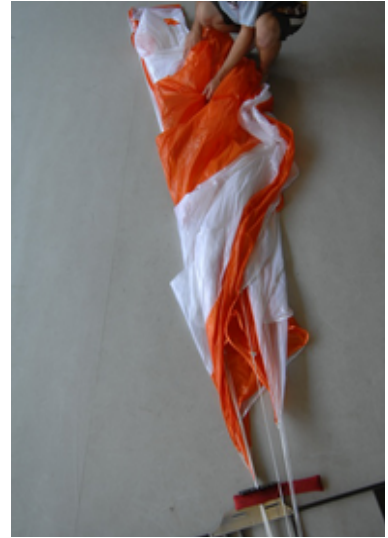
Fig. 63-64 put opposite half of the wing including lines over the line separator to the other side
