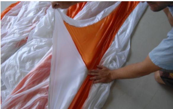
Fig. 36 put the line with its attachment point of panel No. 2 on top of the middle lines and fix it with your hand
