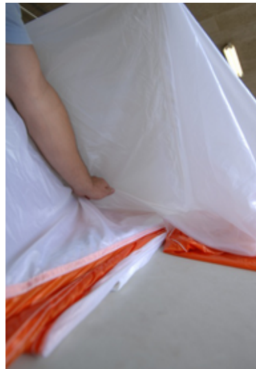
Fig. 42 sweep panel No. 3 outwards (s-fold)
