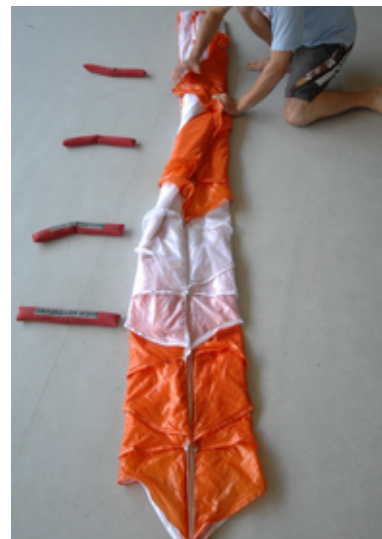
Fig. 79 Put wing sides on top of each other
