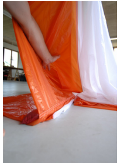
Fig. 51-52 folding of subsequent panels (as far as the wing tip) is carried out according to the description on folding panels 3, 4 and 5
